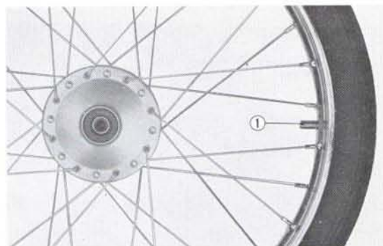
Fig. 4.7 ① Valve stem
